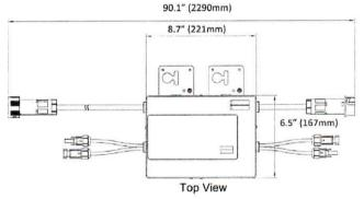
Our flagship product, the APS YC500A is a grid-tied microinverter with intelligent networking and monitoring systems to ensure maximum efficiency. Highly dependable and cost effective, the YC500A handles up to 310W modules with negligible clipping, delivering 250W AC per module with dual MPPT. Half the inverters and half the installation means real cost savings for residential and commercial customers.
