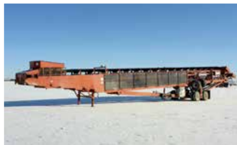
Superior 36X136LP 36 In. x 136 Ft Telescopic Radial Stacking | Grande Prairie, AB, CAN
