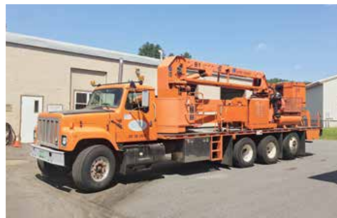
International 2574 w/Aspen Aerials UB50 North Franklin, CT, USA
